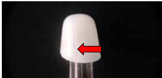
Crack that is made during grinding
